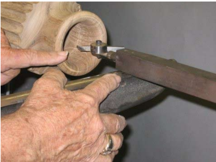
Step 9: Adjust the tool closely to the center line of the rotating wood by moving the tool rest up or down.
