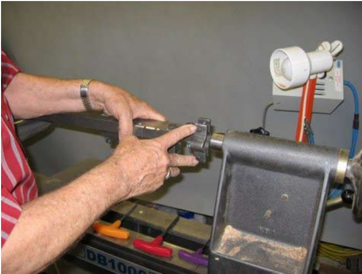
Step 5: Put the clamp over the quill about 1" and snug up the two bolts evenly.
