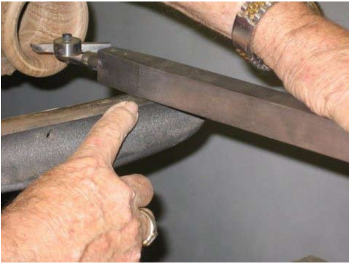
Step 7: Check horizontal tool setting by looking at the tool rest.
