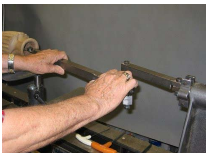
Step 10: Grasp the long bar with both hands and put the cutting edge of the tool into the wood carefully and proceed to remove wood by pulling the tool from the center toward the outer rim.
