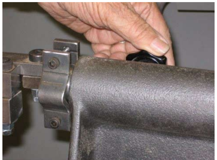
Step 8: While holding the tool horizontal tighten the quill lock.
